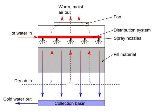
There are many different types of cooling towers but the **cooling tower working priciples** stay pretty much the same. Most cooling towers work based on the principle of "evaporative"
