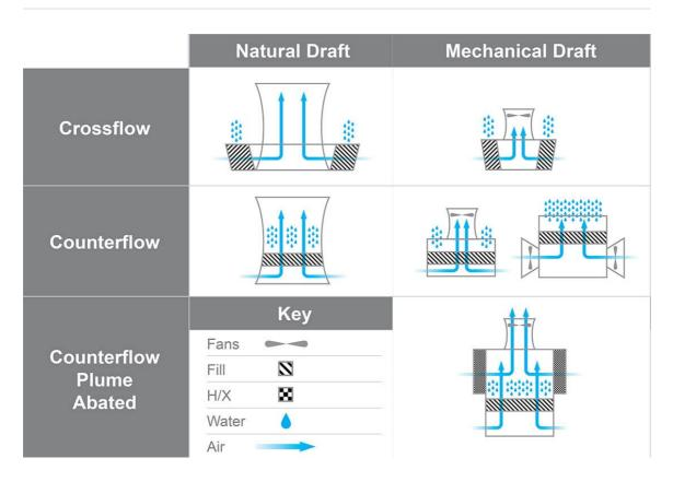
What is a cooling tower? Cooling towers are a special type of heat exchanger that allows water and air to come in contact with each other to lower the temperature of the hot water. During the cooling tower working process, small volumes of water evaporate, lowering the temperature of the water that's being circulated throughout the cooling tower.
