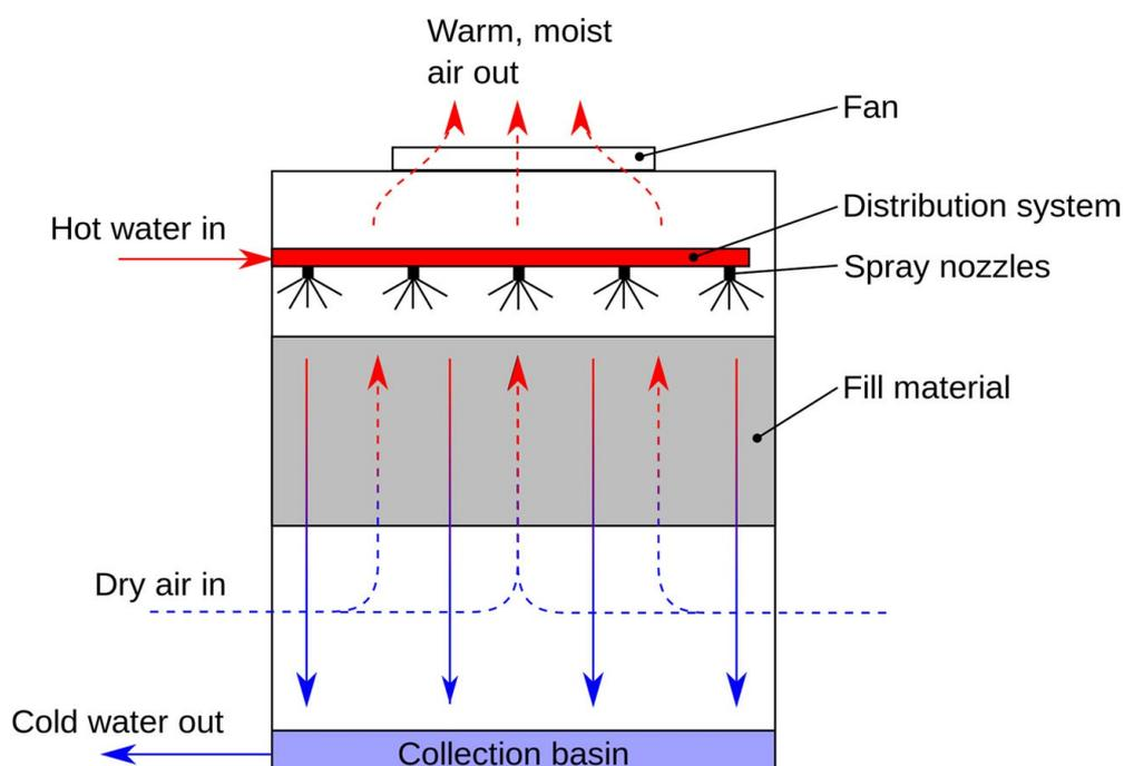
There are many different types of cooling towers but the **cooling tower working principles** stay pretty much the same. Most cooling towers work based on the principle of "[evaporative](#)
